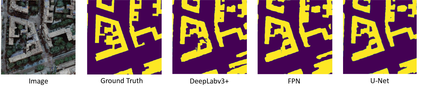
Fig. 3. A comparison of an example image from our dataset and its corresponding ground truth and the predicted mask from three different segmentation models.
