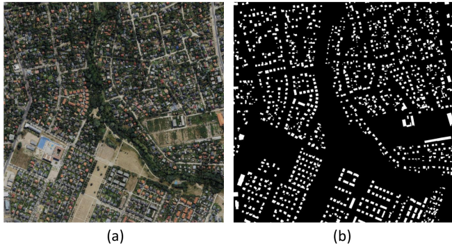
Fig. 2. A sample output pair of the rendering process, depicting an orthographic image render (left) and its corresponding LOD2 model mask (right).
